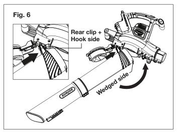
**4.** Insert the collection bag adapter into the blower air outlet until the collection bag is securely fastened (Fig. 7), then clip the bag to the strap holder.
