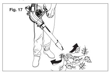
Slowly advance the unit, keeping the accumulated pile of debris in front of you. Most dry blowing operations are better suited to low speeds rather than high speeds. High speed blowing is best for moving heavier items like large debris or gravel.
