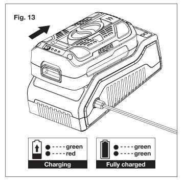
**NOTE:** If the top light remains green while the bottom light alternately flashes red and green, this indicates a temperature abnormality (i.e. that the battery pack is either too hot or too cold). If there is only a red blinking light, this indicates that something is wrong with the battery. Contact Snow Joe<sup>®</sup> + Sun Joe<sup>®</sup> customer service at 1-866-SNOWJOE (1-866-766-9563).
